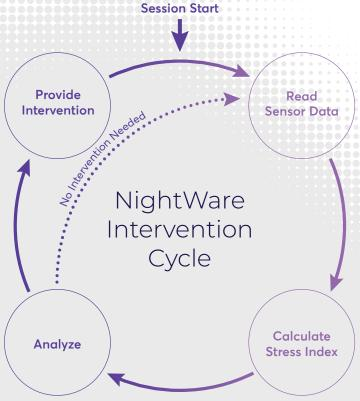
NightWare uses the Apple Watch heart sensor, accelerometer, and gyroscope data to determine if they are having a nightmare.
